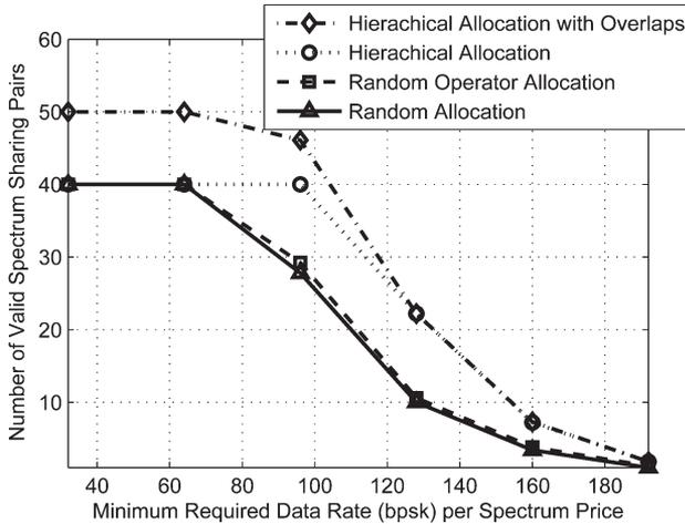
Fig. 6. The number of D2D and cellular or D2D and D2D spectrum sharing pairs for different minimum required data rate (kbits per second) ( $L = 5, K = 100, |\mathcal{J}^i| = 20 \forall i \in \mathcal{O}$ ).
