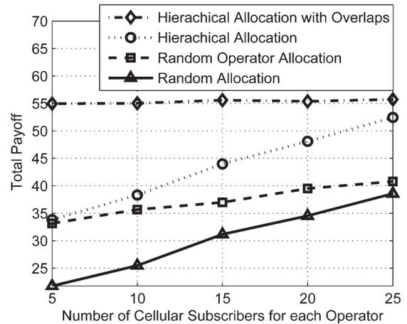
Fig. 8. The total payoff of D2D links for different numbers of cellular subscribers for each operator ( $L = 5, K = 100$ ).
