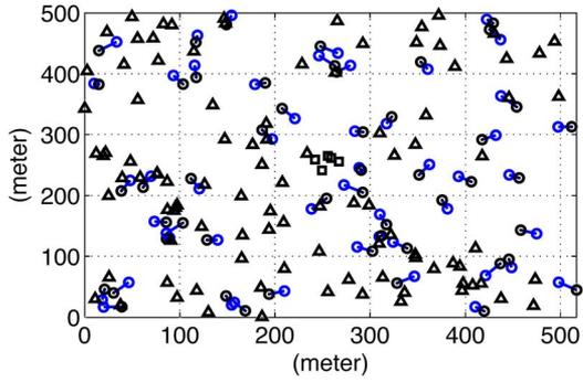
Fig. 3. Simulation setup: we use  $\square$  to denote operators,  $\triangle$  to denote cellular subscribers, blue lines to denote the D2D links, blue  $\circ$  to denote D2D transmitters and black  $\circ$  to denote D2D receivers.
