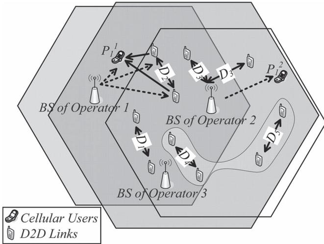
Fig. 1. System model for D2D communications in a cellular network with three operators: D2D links  $D_1$ ,  $D_2$ ,  $D_3$  operate in modes M1 (i.e.,  $D_1$  has been assigned to a dedicate sub-band for exclusive use), M2 (i.e.,  $P_1^1$  and  $D_2$  share the same sub-band) and M3 (i.e., the traffic of  $D_3$  has been forwarded by eNB of operator 2), respectively. D2D links  $D_4$  and  $D_5$  operate in mode M4 (i.e.,  $D_4$  and  $D_5$  share their dedicated sub-bands with each other).
