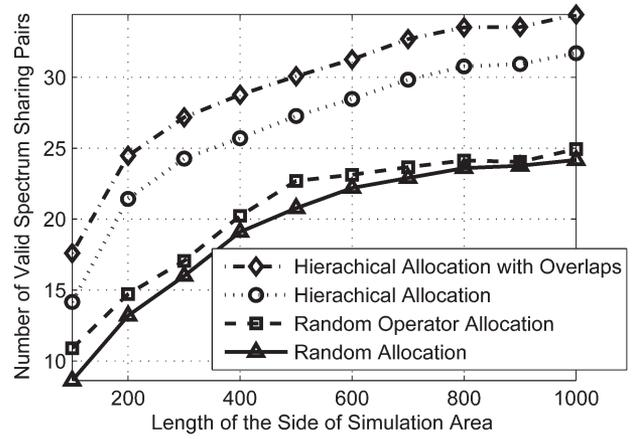
Fig. 5. The number of D2D and cellular or D2D and D2D spectrum sharing pairs for different coverage area sizes ( $L = 5$ ,  $K = 100$ ,  $|\mathcal{J}^i| = 20 \forall i \in \mathcal{O}$ ).
